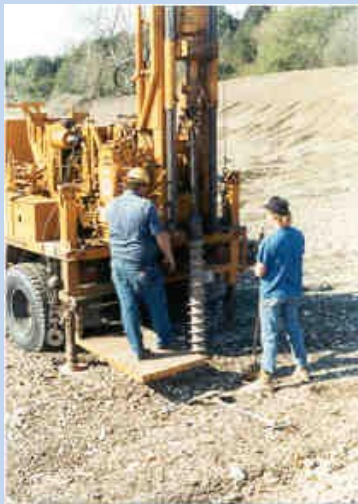
FIGURE 5.3. Hollow-stem auger. (a) Plugged while advancing auger. (b) Plug removed and sampler inserted to sample soil below auger.
