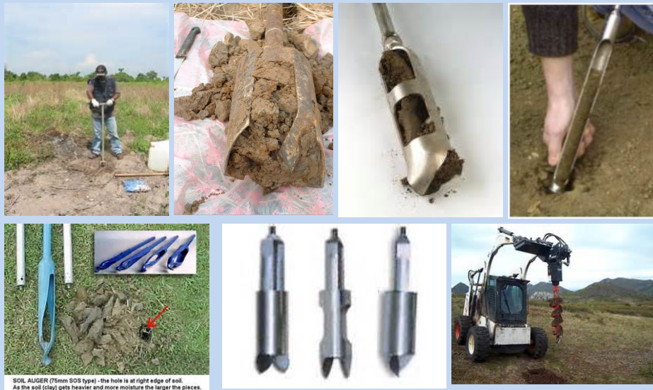
SOIL AUGER (75mm SDS type) - the hole is at right edge of soil. As the soil (clay) gets heavier and more moisture the larger the pieces.
