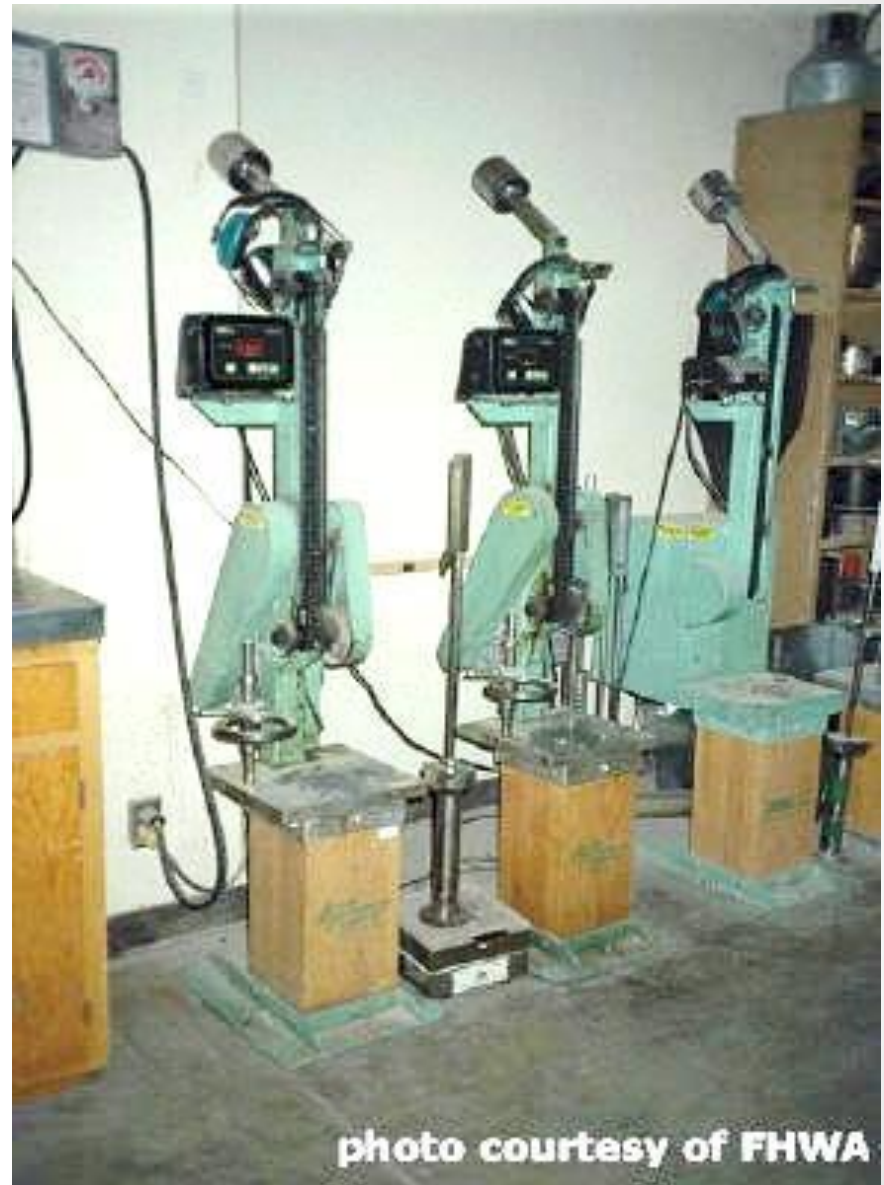
Figure 5.1 – Pedestal, hammer (mechanical) and mold used in preparing Marshall test specimens
