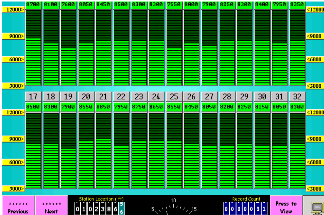
Figure 8.7 – Output from a smart vibrator system showing the frequency of each vibrator
