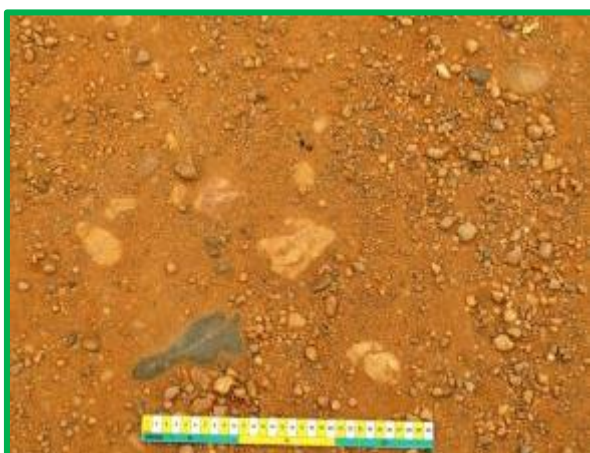
Sub-base mixture of fine hill gravel and coarser alluvium.
