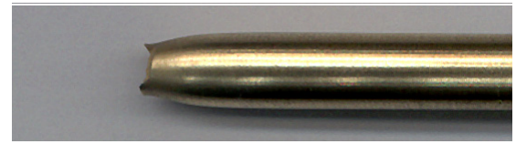
Figure 3.6 Specimen showing necking. (Courtesy Professor J. B. Ligon.)
