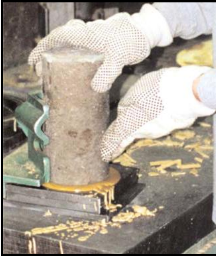
Bonded sulphur capping
