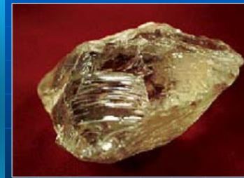
Quartz has a hardness of 7 and shows conchoidal fracture
