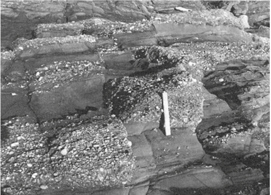
Figure 4.17 Layers of sandstone and conglomerate cut by small faults and joints (some of which are small shears) similar, apart from magnitude of displacement, to the faults. (Reproduced by kind permission of Dr Brian Bluck.)
