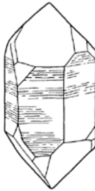
Figure 2.12 A double-ended crystal of quartz. Many quartz crystals in veins are single ended, but all show striations (parallel lines and gouges) across the prism faces.
