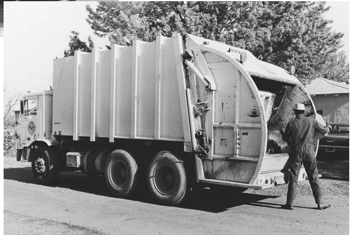
The rear loaded type of collection vehicle is commonly used with two- and three-person crews
