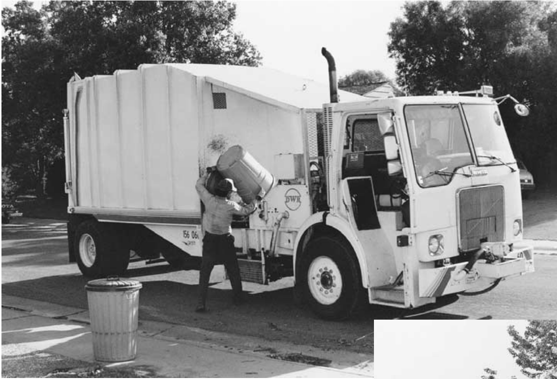
A side-loading vehicle, equipped with a right-hand stand-up drive mechanism
