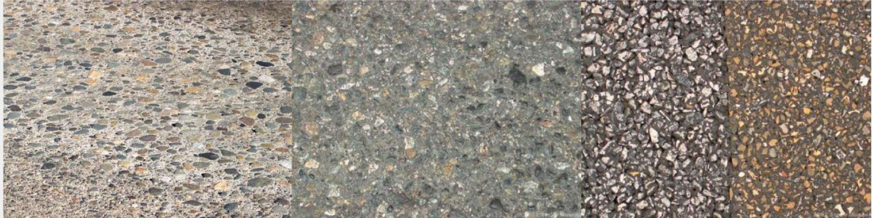
Figure 1: Polished PCC aggregate after 40 years of wear.
