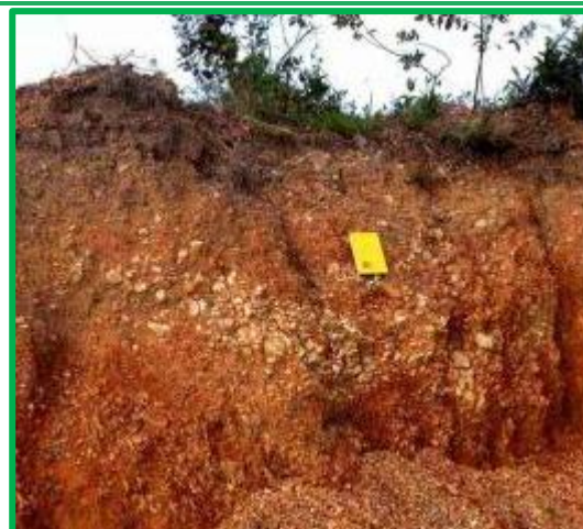
Variability of in situ natural hill-gravel (colluvium)
