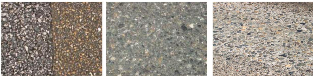
SMAs at the NCAT test track
