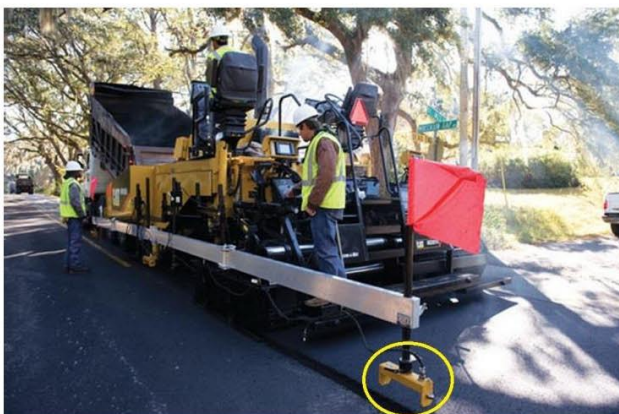
Paver with Sonic Levelling Device
