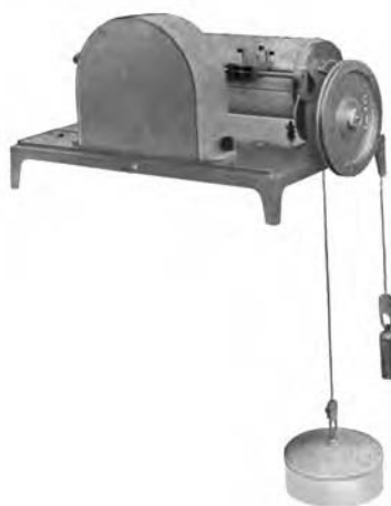
Fig. 4.3 Water-depth recorder — Stevens Type F recorder (Courtesy: Leupold and Stevens, Inc. Beaverton, Oregon, USA)
