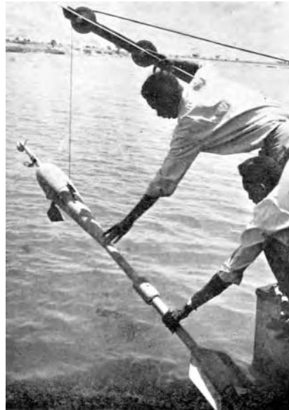
Fig. 4.10 Propeller-type Current Meter—Neyrtec Type with Sounding Weight
