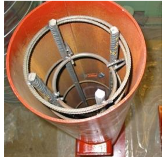
Figure 11 Typical cross-sections of composite columns
