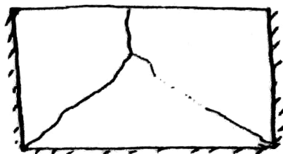
h) Fixed supports on three sides
