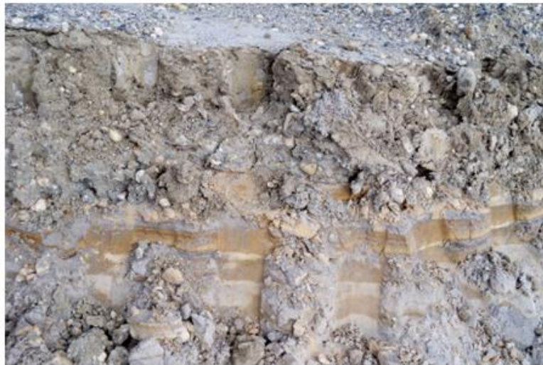
This is a 4 ft cross section of the sandy surface sediment of marine origin. Visible layers containing calcium phosphate, quartz & other minerals.
