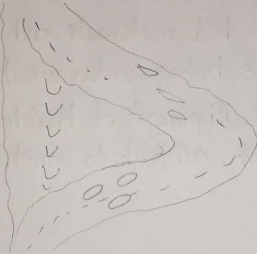
Fig: Development of a chute cutoff.
