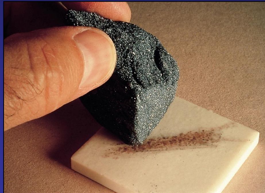
Hematite (Fe 2 O 3 ) can have various colors, but its streak is always red-brown
