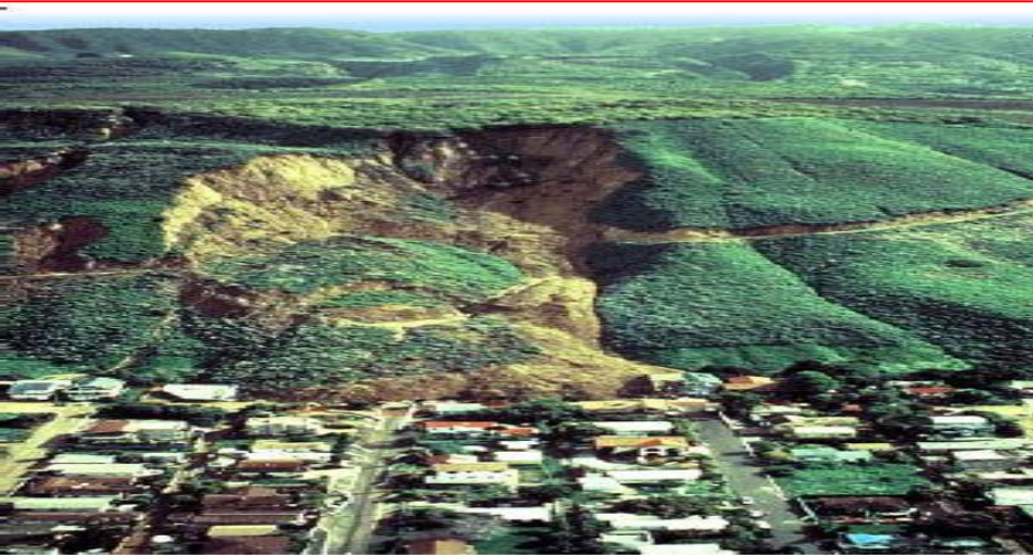
C. Slide Shear failure causing slump to more stable configuration.
