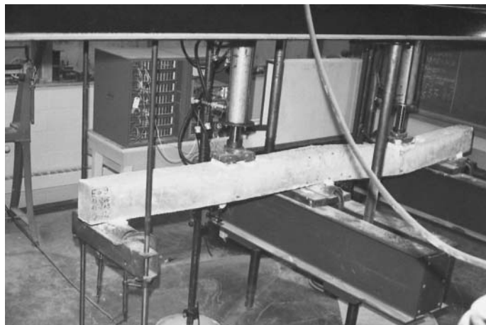
Two-span continuous reinforced concrete beam loaded to failure.
