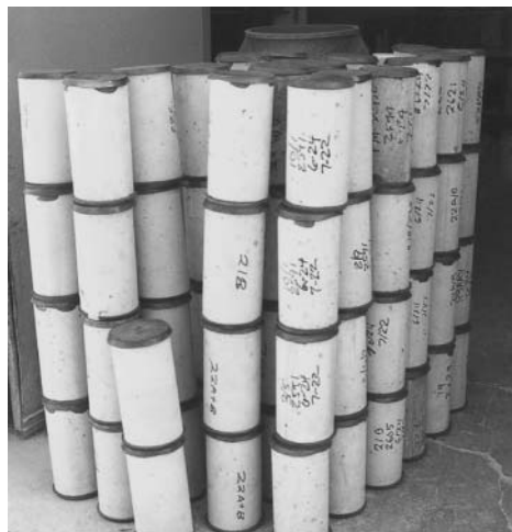
Standard capped cylinders ready for testing.
