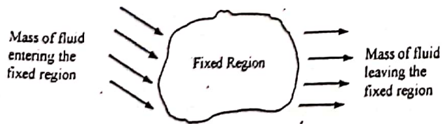
Fig. 4.18 Diagrammatic Representation of the Principle of Conservation of Mass
