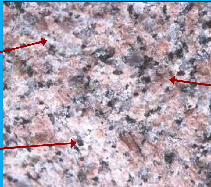
Granite rock with a phaneritic texture
