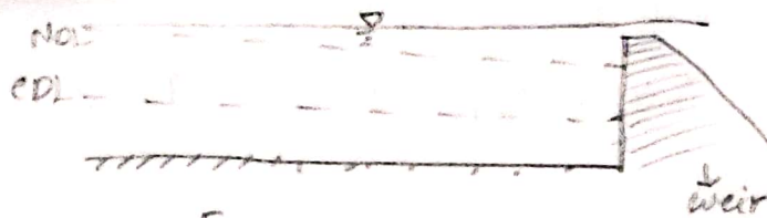
Fig: Flow behind a weir
