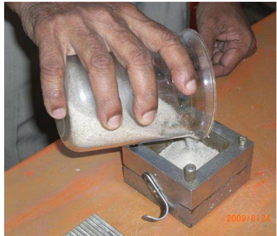
Preparation of a sand specimen
