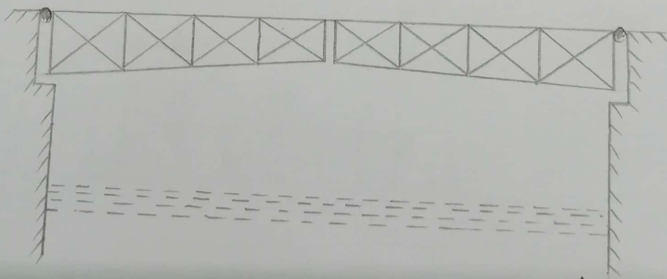
Fig 1.12: Double Bascule Bridge.
