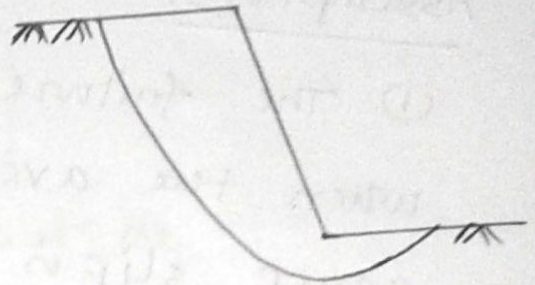
(c) Base failure.
