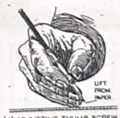
Fig. 2.65 Position of Hand in Using the Ruling Pen.
