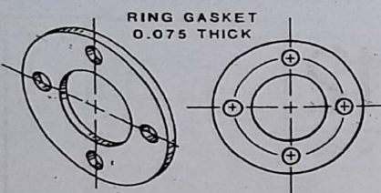
FIG. 12-2 Single view for flat objects
