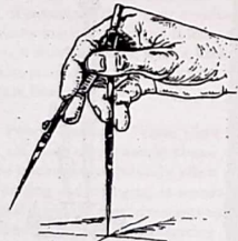
Fig. 2.48 Adjusting the Dividers.
