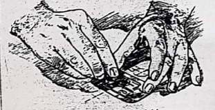
Fig. 2.18 Using the Erasing Shield.
