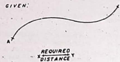
Figure 3-22A How to draw a line parallel to a curved line at a given distance
