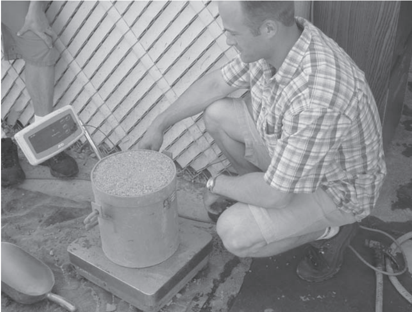
FIGURE A.29 Weighing the aggregate.
