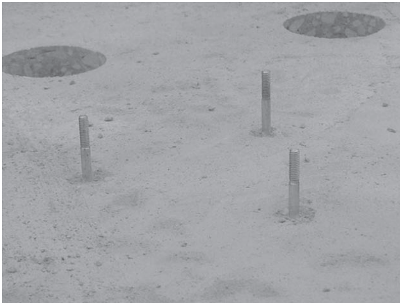
FIGURE A.49 Three probes driven into concrete.
