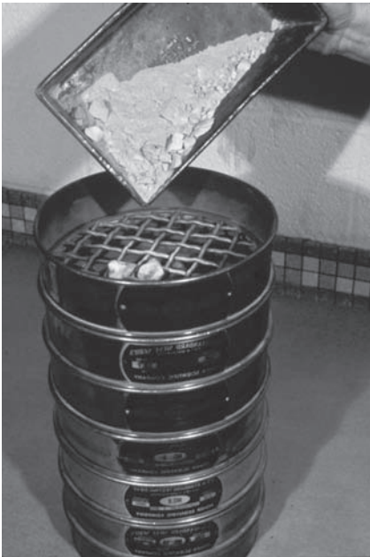
FIGURE A.22 Placing aggregate sample in the sieves before sieving.
