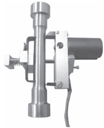
FIGURE A.7 Extensometer attached to a steel specimen. (Courtesy of Instron®)
