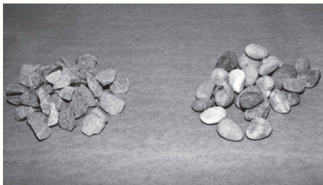
FIGURE 5.4 Angular and rounded aggregates.
