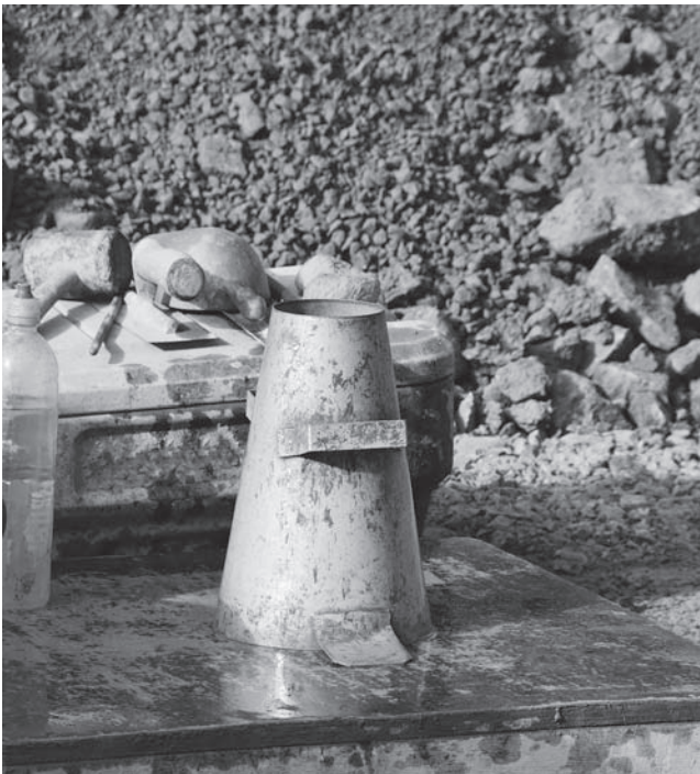
FIGURE 7.4 Slump test apparatus. (Fotolia/Bradlee Mauer)
