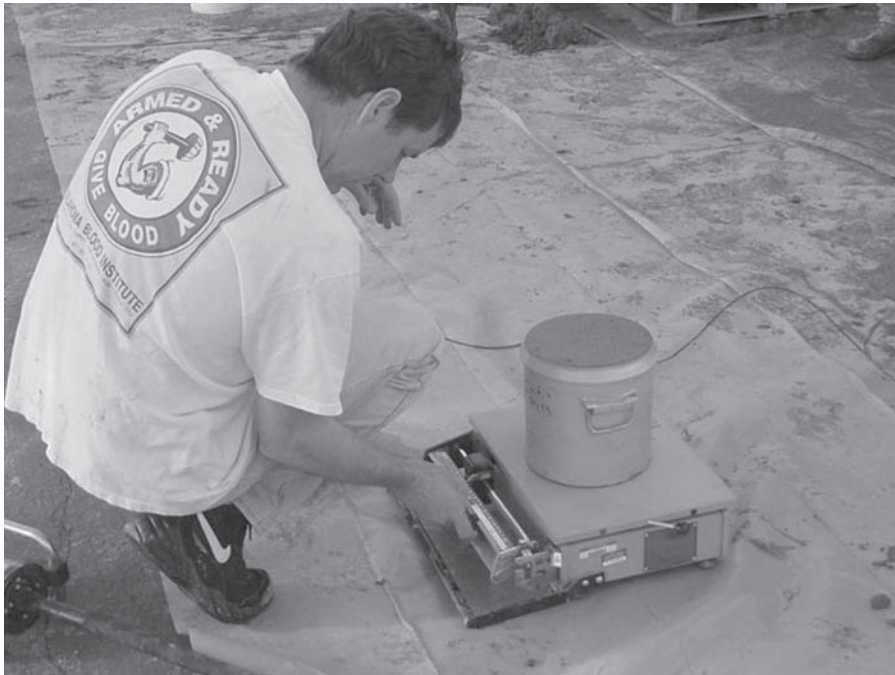
FIGURE A.33 Weighing concrete inside the container.
