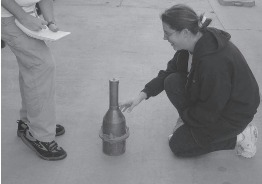
FIGURE A.35 Reading air meter.
