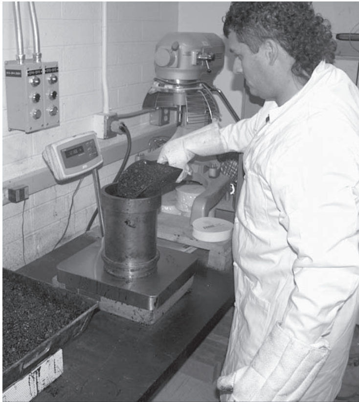
FIGURE A.57 Placing HMA in mold.
