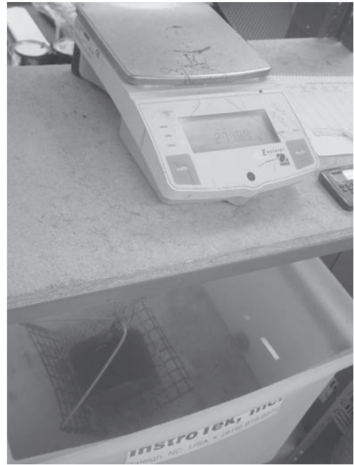
FIGURE A.65 Weighing HMA specimen in water.
