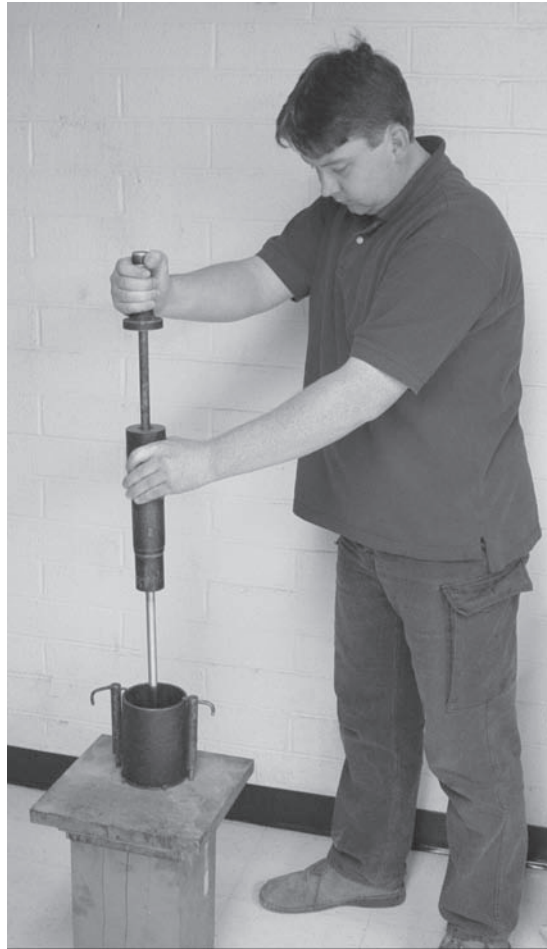
FIGURE A.61 Compacting an HMA specimen using a manual Marshall hammer.
