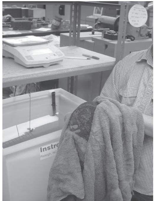
FIGURE A.65 Weighing HMA specimen in water.
