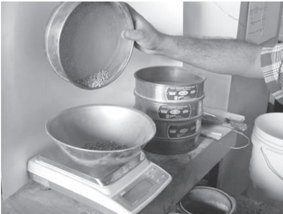
FIGURE A.23 Weighing aggregate retained in sieves.
