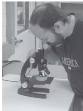
FIGURE A.16 Viewing concrete specimen with an optical microscope.
