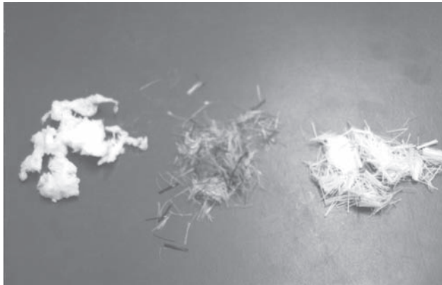
FIGURE 7.51 Fibers used for fiber-reinforced concrete.
