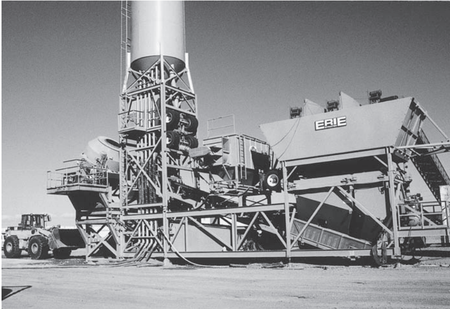
FIGURE 7.6 Mobile batcher mixer at the job site.
