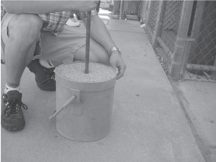
FIGURE A.28 Rodding aggregate in the container.
