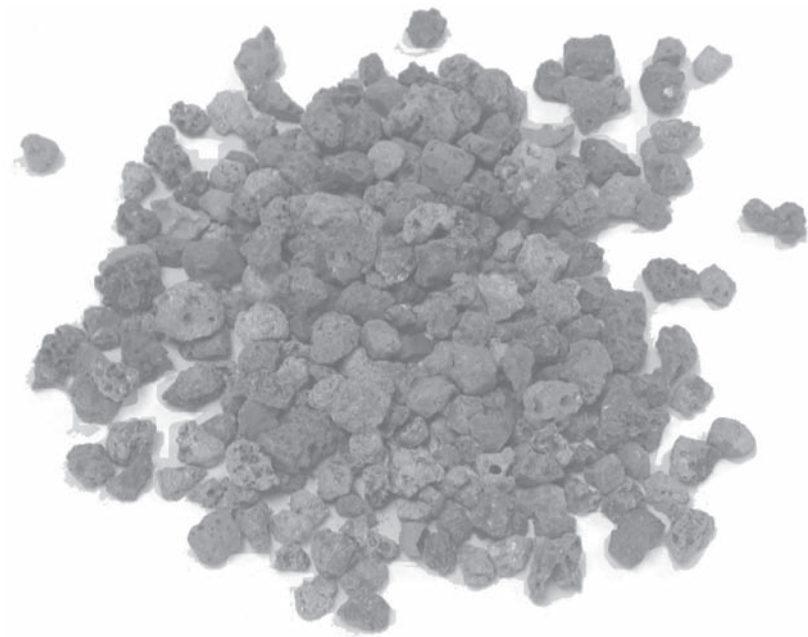
FIGURE 7.48 Aggregate used for lightweight concrete.
