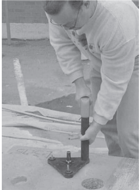
FIGURE A.48 Firing and driving Windsor probe into concrete using triangular positioning device.
