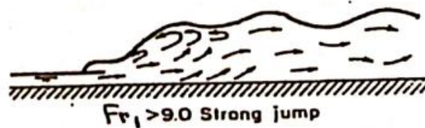
Fig. 7.2 Hydraulic jumps in horizontal rectangular channels
