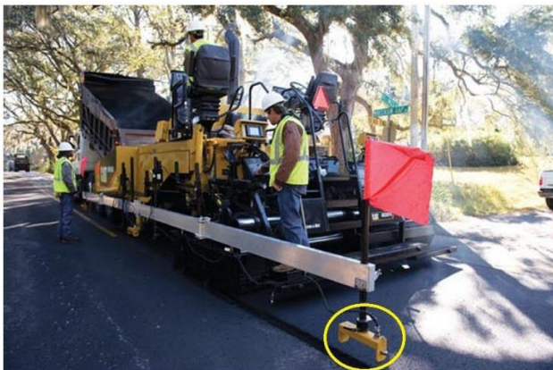
Paver with Sonic Levelling Device
