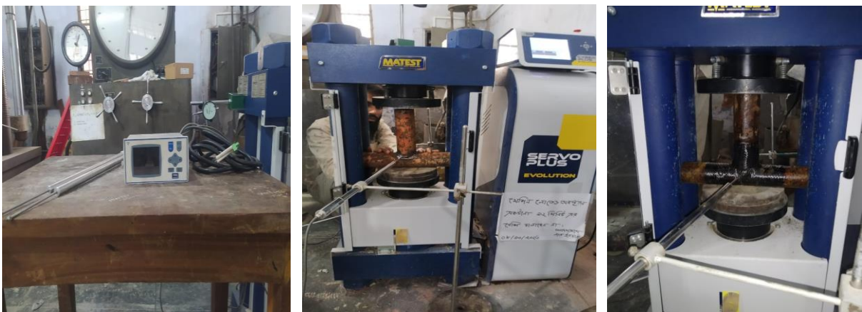
Figure 6: Specimens testing under CTM and LVDT
