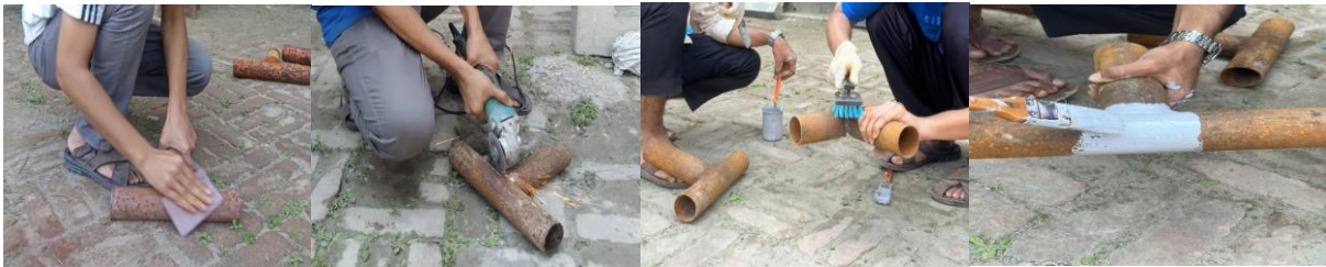
Figure 4: Specimens smoothing, cutting, brushing and applying primer
