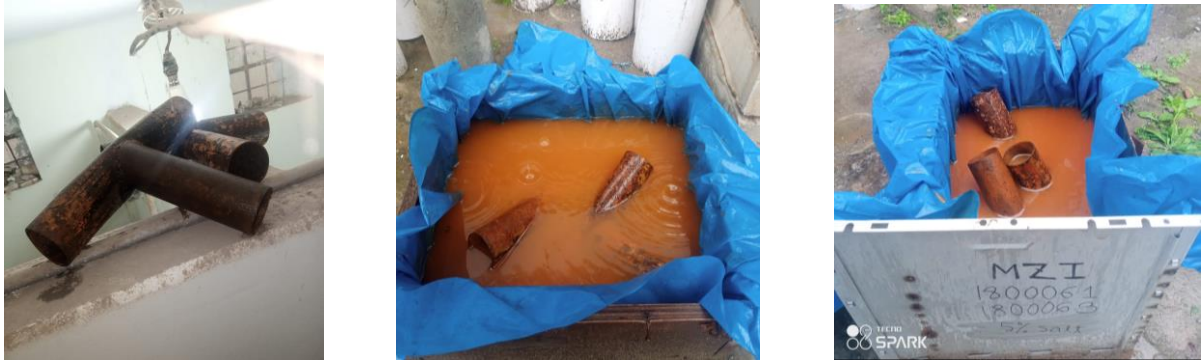
Figure 3: Specimens under humid, cyclic rain water and cyclic 5% salt water condition
