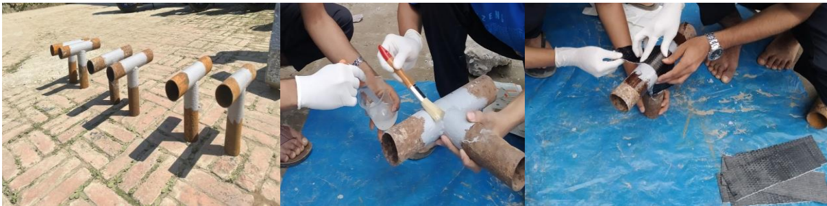
Figure 5: Specimens drying, application of adhesive and CFRP wrapping
