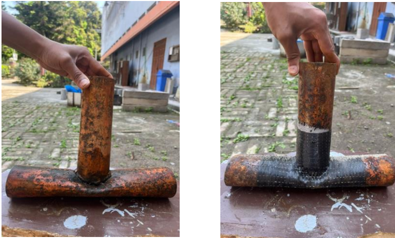
Figure 7: Deformed specimens after applying load
