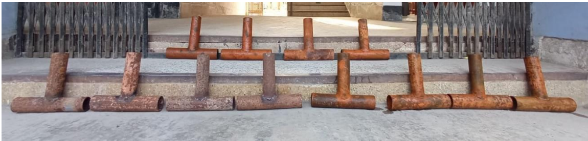
Figure 1: Total 12 specimens of corroded tubular T-joints for experiment
